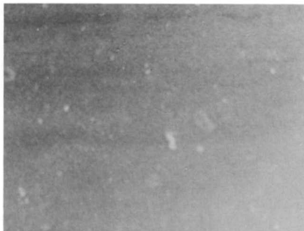
Figure 15 Scanning electron micrograph of 67PVA/33HEMA (2% GLA, 2% BDDMA). (Magnification \times 1447 )
